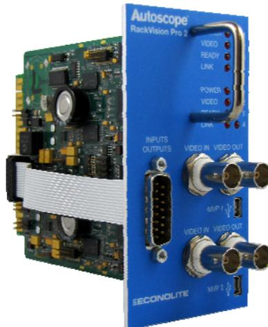
*The Autoscope RackVision Pro 2 video vehicle detection system meets the attached specifications.*
